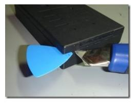
The sides went apart easy ... but at the bottom the case had a better connection. I used two prying tools and pushed them right till the bottom. With patience and a little force (tilt the upper part towards the bottom) the case snapped apart.
