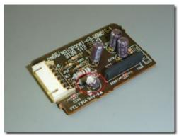
Some further investigation showed, that there is a capacitor (2278) attached to the DC offset line that should flatten all the AC signals. When I measured the capacitor with the LCR-Meter there was no reading of the capacitance possible (the capacitor was dead). I replaced the capacitor with a new one with the same values (I used a 105 °C rated) and did the first measurement (with 0° phase shift) once more.
