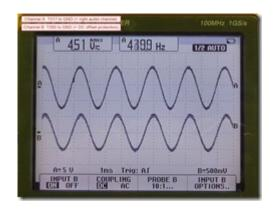
The protection circuit has a TA7317P IC in it. If you look at the datasheet you see that the IC will send the amplifier to protection mode when a voltage level of approximately 1 V is exceeded. With this information it seems plausible that (given the signal at T050 as shown above) the amplifier switches to protection mode.
