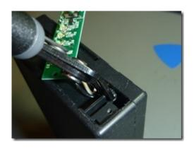
The next step is the most time consuming. You have to cut around the case where the upper and the lower part have been welded together. I used a cutting blade and repeatedly cut along the edge.
