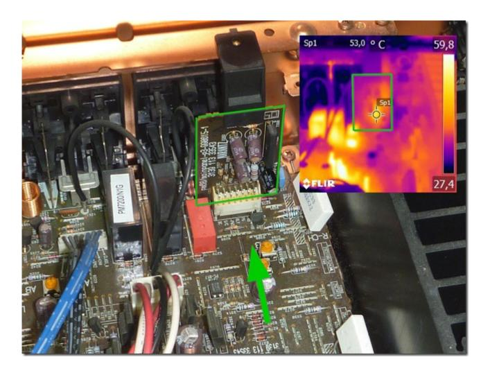
I did some thermal imaging of the protection circuit board. The picture above was taken after 5 minutes idle time of the amplifier (switched on but no signal). The green arrow indicates the approximate direction of the IR Image. The green frame marks the protection circuit board. As you can see there is a hotspot (53 °C) very close to the broken capacitor caused by two 1 W resistors (3364 and 3358). The permanent exposure to heat probably killed the capacitors.
