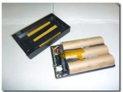
Don't stick on the top cover of the battery pack right now. There would be a small gap where we cut the case apart.
