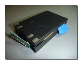
There are 6 single sub C cells that are joined in serial.
