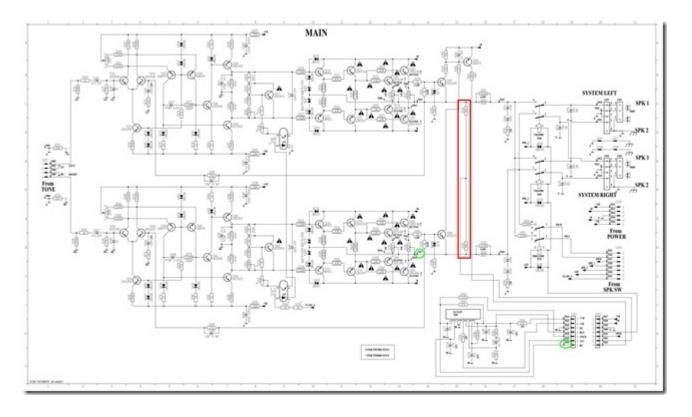
If you search on the internet, you can find a service manual which is really helpful because it has all the schematics in it. Because all the signals I measured so far seemed fine, I decided to investigate the protection circuit and measure the signals there. By studying the schematic of the main amplifier one can see, that at the end of the output stages the signal gets tapped of to the protection circuit (marked with the red
