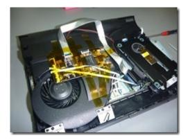
You also have to connect the small cable to the cover switch. Because of the placement of the PCB (I don't think there is a better place) the cable provided are hardly long enough. To install the cover switch cable I lifted the optical drive out of its position a bit closer to the PCB. After connecting the cable you can put the drive carefully back. You will see that the cable is under a bit of tension, but I think it will do. The position of the larger cable is not fixed yet.
