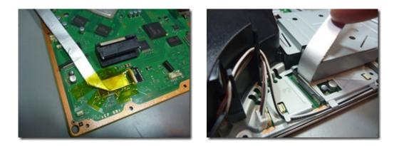
The power cable installation is documented in the manual. Be careful to plug the cable in the right way. The tapping where the small cables are need to be on the power supply side. I did it wrong the first time (the PS will not turn on). The In the picture below you can see the position in which I mounted the ODE V5.10b. Additional to the double sided tape I secured
