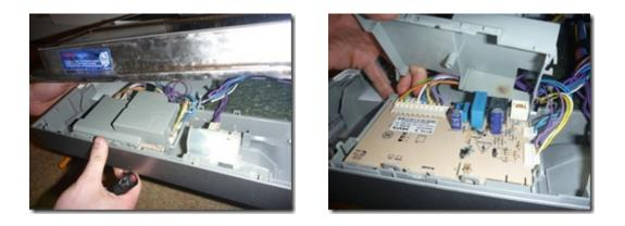
To remove the front, open the dishwasher and undo the screws that are on the inside of the front door. The two screws in the middle hold the wood faceplate. You don't need to take the faceplate off, but It makes the handling a bit easier (however to mount it back on it is good to have someone that helps you).
