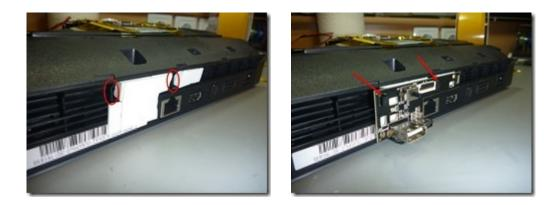
After that you can install the two cables. I secured them firmly with Kapton. The last thing to do is to attach the power cable and fixate it.
