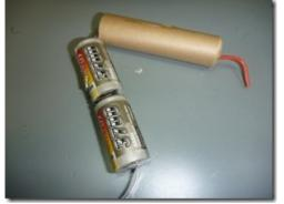
To fixate the new battery pack in the cover I used very thin double side adhesive tape (some Tesa that is usually used for sticking photos to an album).
