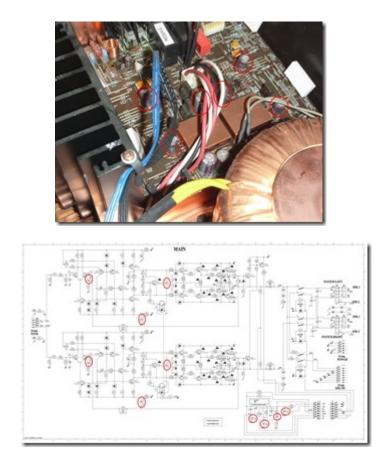
In the schematic above I marked all the components that I replaced. If you replace them, be sure to use 105 °C rated capacitors. The capacitors of the power supply where ok so I didn't replace them. Be sure to do a DC offset voltage alignment and an idling current adjustment after you replace those components. At my unit the values have drifted a bit. You find detailed instructions on how to perform this adjustment in the service manual at page 34.
