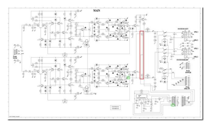
If you search on the internet, you can find a service manual which is really helpful because it has all the schematics in it. Because all the signals I measured so far seemed fine, I decided to investigate the protection circuit and measure the signals there. By studying the schematic of the main amplifier one can see, that at the end of the output stages the signal gets tapped of to the protection circuit (marked with the red box). This signal is for DC offset detection.
