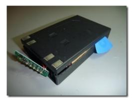
There are 6 single sub C cells that are joined in serial.
