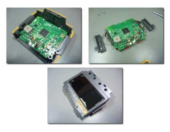
After you removed the PCB from the housing the display is still connected to the PCB. You have to pry open the red
