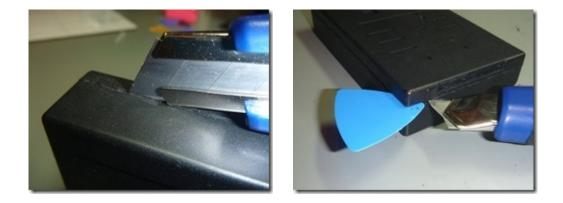
The sides went apart easy ... but at the bottom the case had a better connection. I used two prying tools and pushed them right till the bottom. With patience and a little force (tilt the upper part towards the bottom) the case snapped apart.
