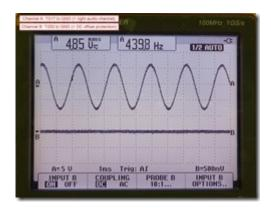
As to be expected the signal at T050 changed drastically. All the AC part was gone and the amplifier didn't turn off anymore! Yeah ... problem found and fixed! To be safe I replaced all four electrolytic capacitors (2278, 2281, 2282, 2279) on the protection board. I measured them later on and they all where in pretty bad condition.
