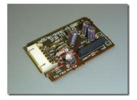
Some further investigation showed, that there is a capacitor (2278) attached to the DC offset line that should flatten all the AC signals. When I measured the capacitor with the LCR-Meter there was no reading of the capacitance possible (the capacitor was dead). I replaced the capacitor with a new one with the same values (I used a 105 °C rated) and did the first measurement (with 0° phase shift) once more.
