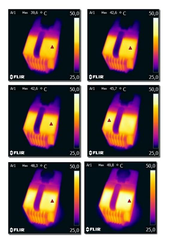
After tree hours the temperature was steady and didn't increase any more. The room temperature was at about 24°C.
