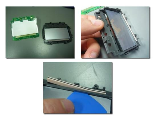
In order to change the LCD you have to lift it slightly up and slide it out in the directions of the buttons. At my unit the conductive rubber zebra stripe was stuck to the PCB. I used a pick to separate it carefully.
