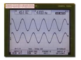
The protection circuit has a TA7317P IC in it. If you look at the datasheet you see that the IC will send the amplifier to protection mode when a voltage level of approximately 1 V is exceeded. With this information it seems plausible that (given the signal at T050 as shown above) the amplifier switches to protection mode.
