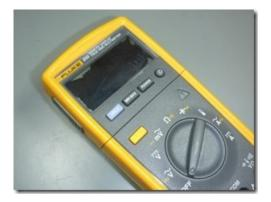
The special thing about this meter is, that you can separate it into the base unit and the display unit. They communicate by wireless transmission up to 10m.
