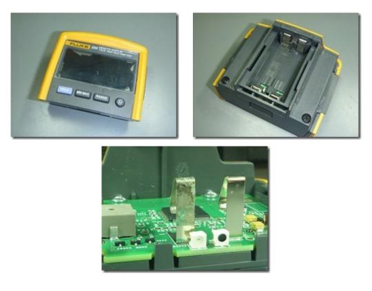
On two of the battery terminals there was a bit of corrosion. Probably someone had left batteries to long in there. With a screwdriver and some alcohol prep pads the dirt came off really easy.
