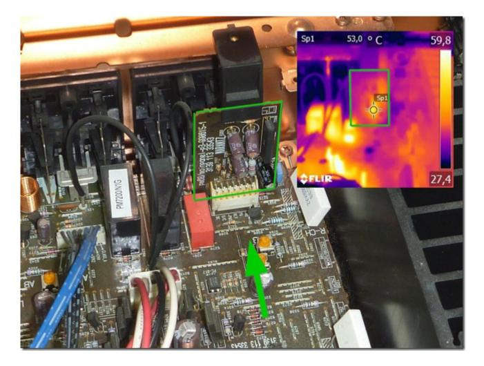
I did some thermal imaging of the protection circuit board. The picture above was taken after 5 minutes idle time of the amplifier (switched on but no signal). The green arrow indicates the approximate direction of the IR Image. The green frame marks the protection circuit board. As you can see there is a hotspot (53 °C) very close to the broken capacitor caused by two 1 W resistors (3364 and 3358). The permanent exposure to heat probably killed the capacitors.
