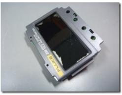
After you removed the PCB from the housing the display is still connected to the PCB. You have to pry open the red marked plastic clips gently. The LCD assembly will then come off.
