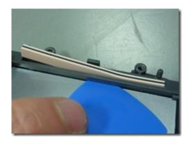
In order to change the LCD you have to lift it slightly up and slide it out in the directions of the buttons. At my unit the conductive rubber zebra stripe was stuck to the PCB. I used a pick to separate it carefully.
