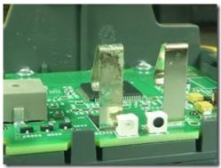
On two of the battery terminals there was a bit of corrosion.
