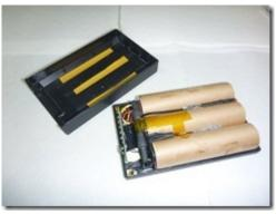
Don't stick on the top cover of the battery pack right now. There would be a small gap where we cut the case apart.
