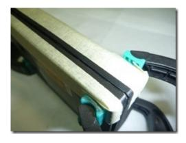
Apply a small amount of the construction silicone around the edge of the lower case. Don't use to much or it will get messy once you put the case together. If it really is too little (trust me there wont) you can apply more when the case is put together.
