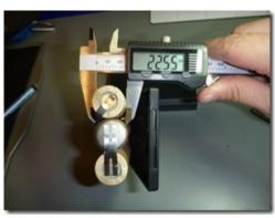
The six batteries are all wired in series  $(6 \times 1,2V = 7,2 \ V)$ . The two batteries in series are 86mm long and have a diameter of 22,5mm.
