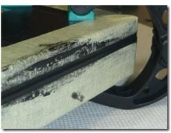
Let it dry for at least 24 hours (depending on the type of silicone you used). After drying you can remove the tape.
