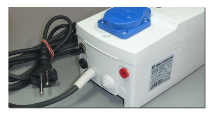
The Breve-Tufvassons PFS 250 is an isolation transformer I bought on ebay. It is a small unit that can be easily carried. Whenever I repair things on the go, I take that little unit with me. Just the extra bit of security so that I feel comfortable when working on mains powered devices.
