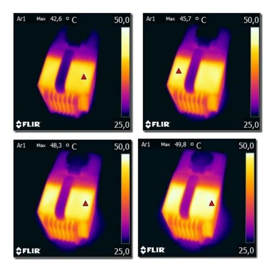
After tree hours the temperature was steady and didn't increase any more. The room temperature was at about 24°C.
